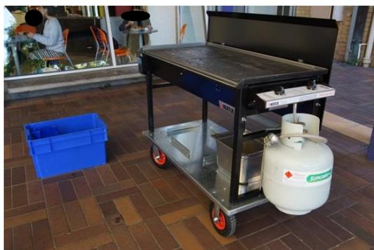
11. Connect gas line / safety valve to the gas cylinder (which should remain on the hooks) with the black knob. Note that the attachment is a left hand thread – therefore screw anti-clockwise to attach. Take care not to cross thread the attachment and hand tighten firmly.
